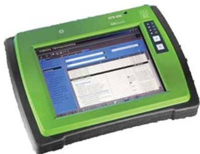
Figure 2 With the help of Kontron MARS, mobile applications - such as the diagnostic system for automobiles shown here - can be supplied with an uninterrupted flow of power: A fall back battery allows to replace the discharged battery without intermission.
