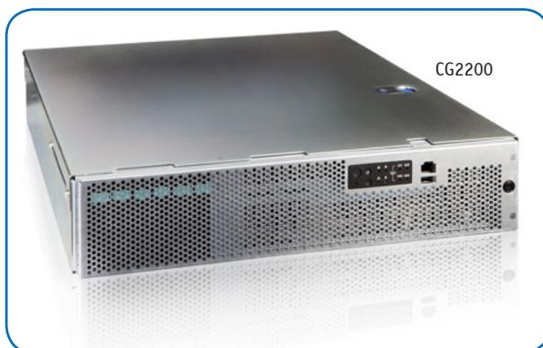
In contrast to standard enterprise style servers the CG2200 has been designed to withstand extreme heat, humidity, altitude and zone 4 earthquake shock and multiple other extreme environmental conditions in compliance with NEBS-3/ETSI requirements. Also important for the rigid requirements of the telecom central office, the server includes advanced server management and Telco alarm management features that provide visual, audible (optional) and SNMP event indications of faults.
